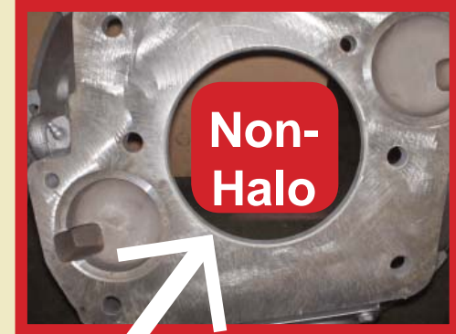
Back of Bell Housing is flat
