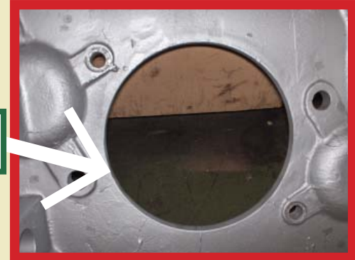
Front of Bell Housing is flat
